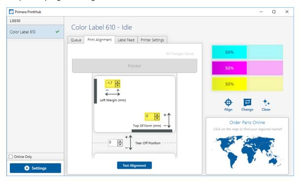
**Note:** It is best to over bleed as little as possible to avoid excess ink on the label backing. Also, over bleeding too much will cause the Printer to skip labels. This is because the Printer stops printing too late to sense the next label.
